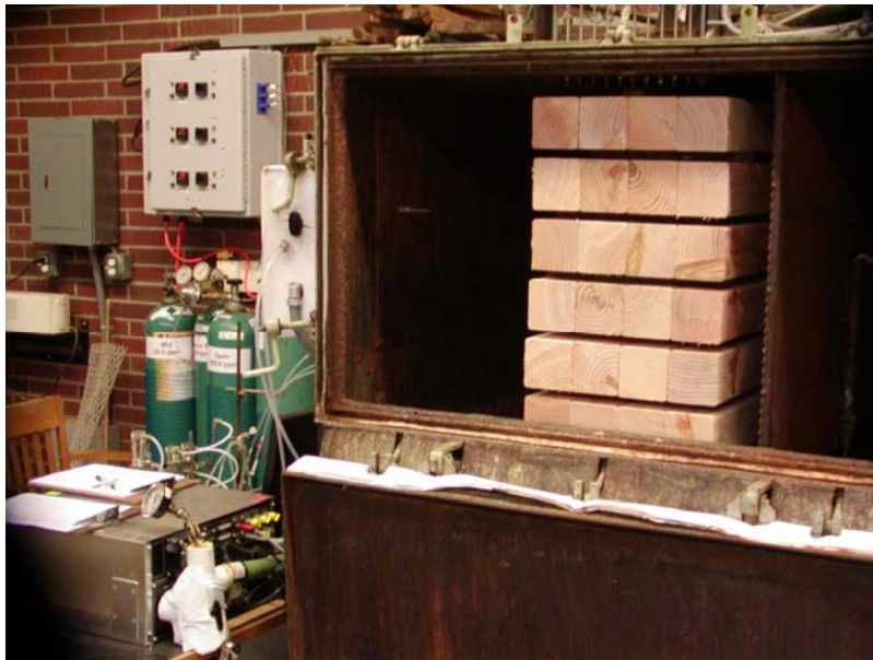
FIGURE 7. Schematic of kiln and sampling system (top) and photo of kiln loaded (bottom).
