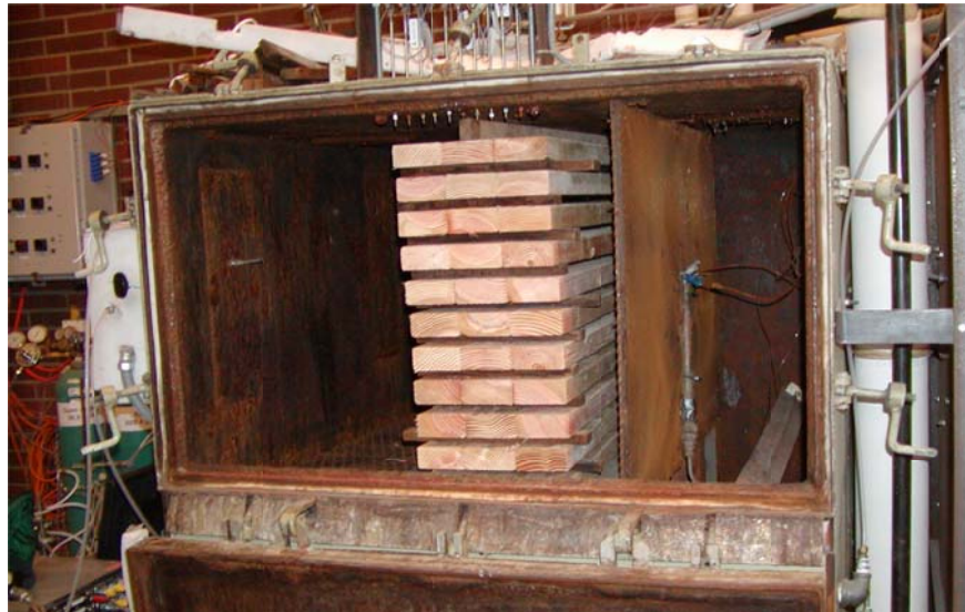
Figure 7. Schematic of kiln and sampling system (top) and photo of kiln charge (bottom).
