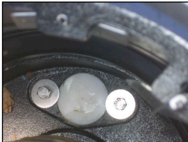
Figure 1-4 1DP-2100 Field Installed Drain Plug
